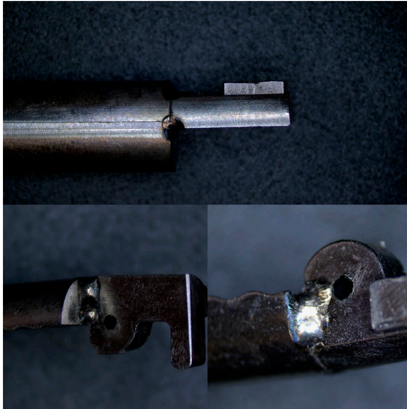
Figure 16. Gripper laser welding results
