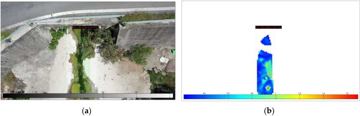
Figure 10. The studied section of Agra captured by the UAV (a) the vectors of velocity are depicted in green color; (b) the vectors of velocity are depicted in a colorized scale where dark blue corresponds to 0 and yellow to >0.8 m/s.
