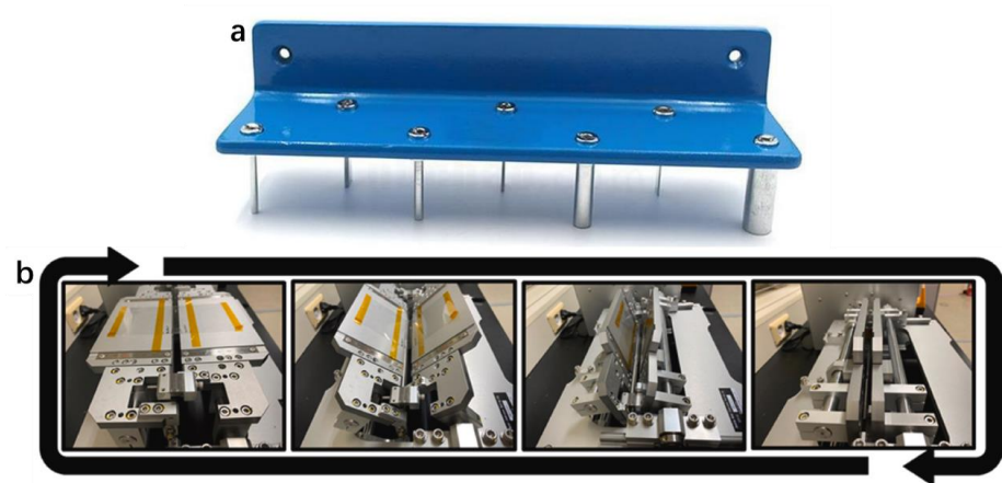
Figure 6. (a) Flexibility tester [73], coatings were deposited on tinplate and bent on shaft rods of different diameters in this method. The flexibility was determined by the minimum diameter of the shaft rod that did not make the coating crack after bending [50]. (b) Photograph of the dynamic bending test. Reprinted with permission from Composites Part B: Engineering [13]; Copyright 2022 Elsevier.
