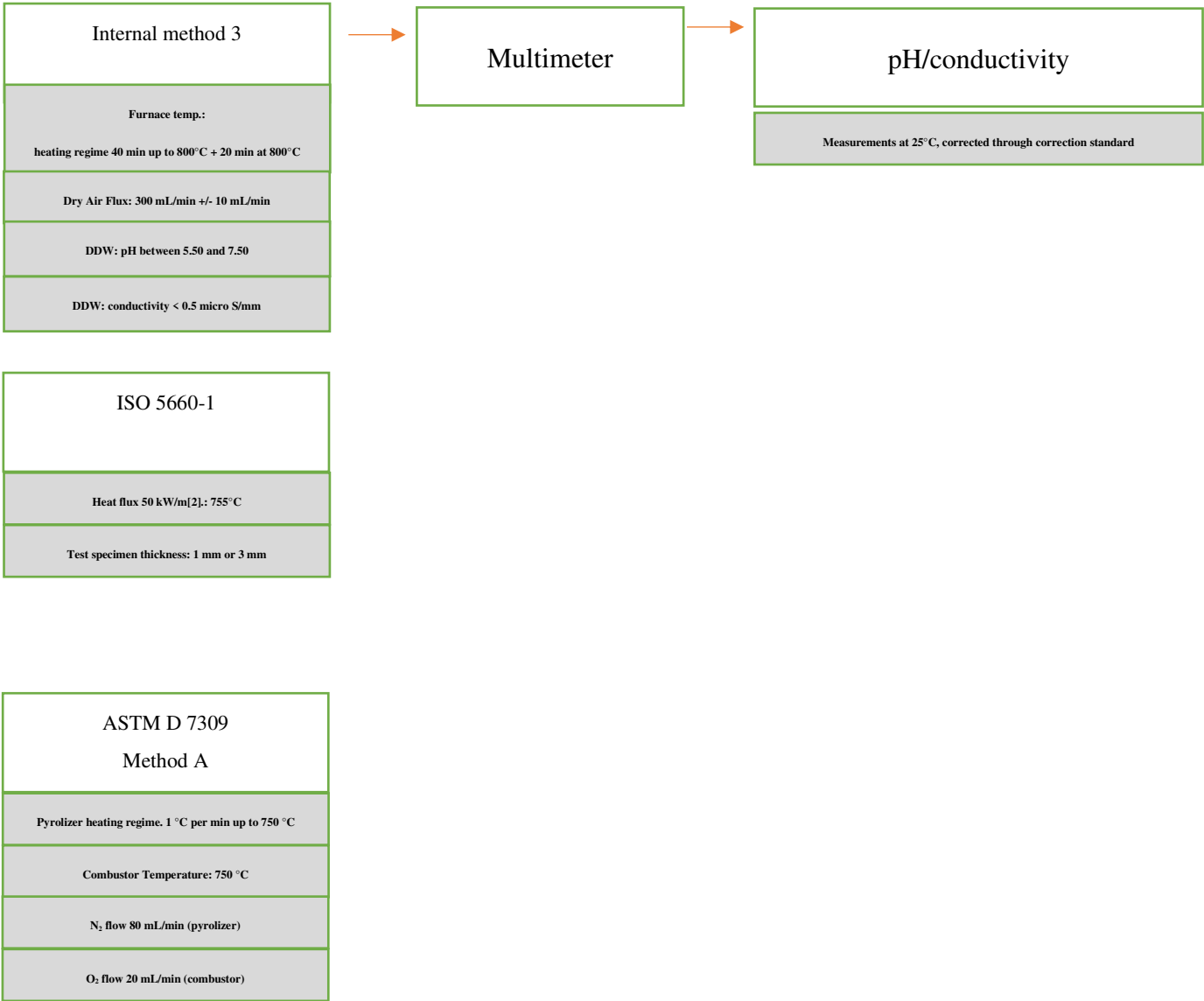
Figure A2. A schematic diagram of the testing process and main conditions.
