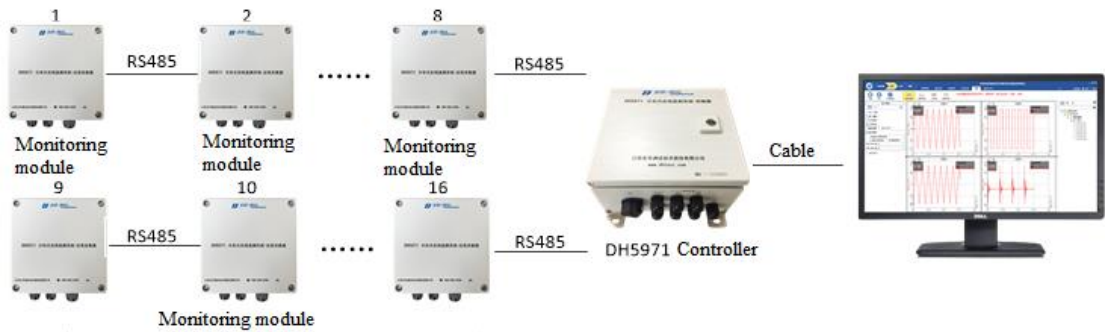
Figure 5. Diagram of connecting the DH5971 distributed online monitoring system.
