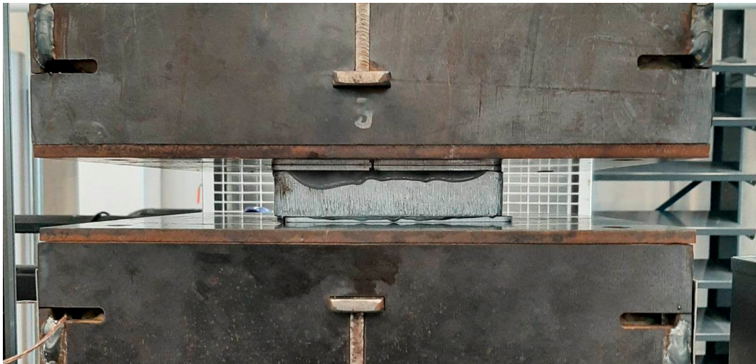
Figure 5. Compressed mold demonstrated by visible flash and sealed lid to mold body.
