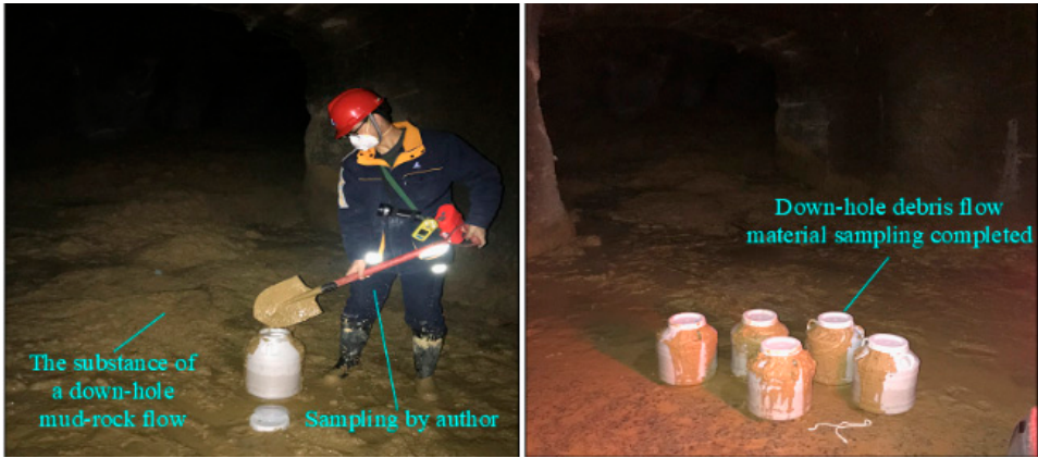
Figure 5. Field sampling of debris from the Plan mine.
