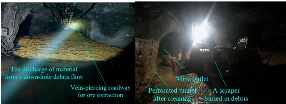
Figure 2. Map of the debris flow accident in Plan copper mine.
