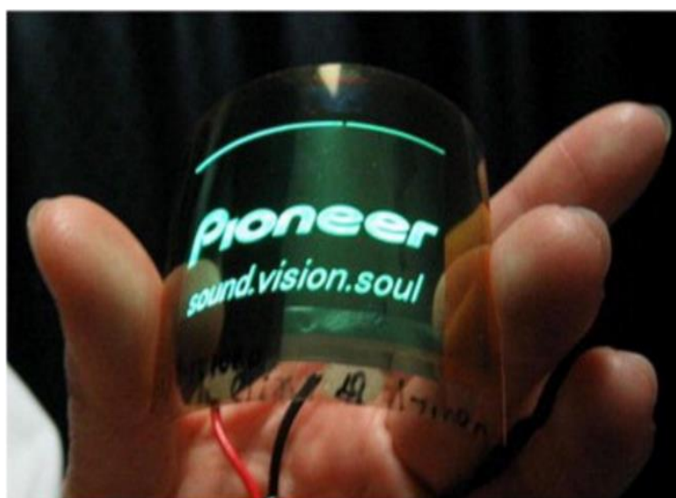
Figure 23. Flexible display on CNF substrate [250]. [Reused with permission from publisher].
