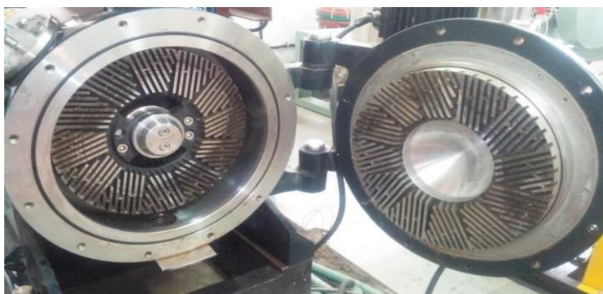
Figure 8. Disc refiner opened to show the refining surfaces [78] [Reused with permission from publisher].
