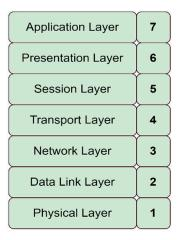
Figure 1. OSI model layers (client side top to bottom; server side bottom to top).
