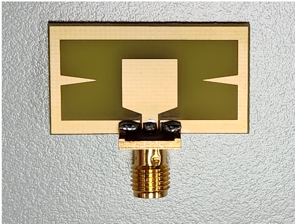
Figure 10. The prototype of the proposed antenna with an SMA connector soldered to it.
