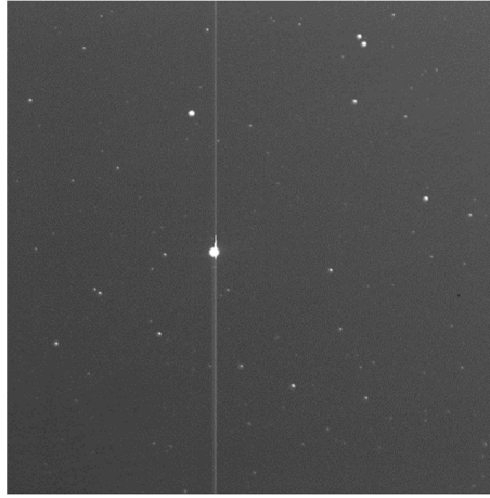
Figure 4. Excessive stellar energy leads to electron overflow after extending the integration time.
