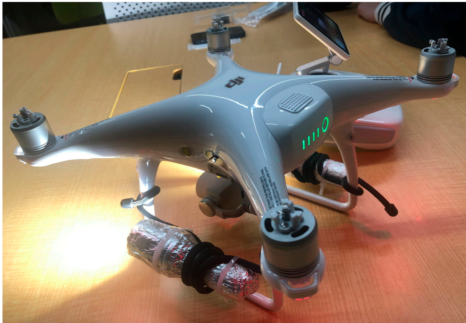
Figure 18. Wrapping the light in aluminum foil.
