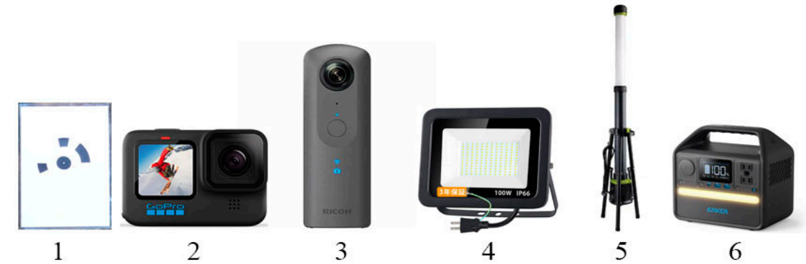
Figure 4. Equipment for creating 3D models in dark environment 1, 1. Ground Control Point 2. Normal camera (GoPro Black Hero 10) 3. 360-degree camera (Ricoh Theta 360) 4. Normal LED light (10000 Lumens LED) 5. Omni-directional LED light (Tube 10000 360-degree LED (10000 Lumens) 6. Anker 100w portable battery.
