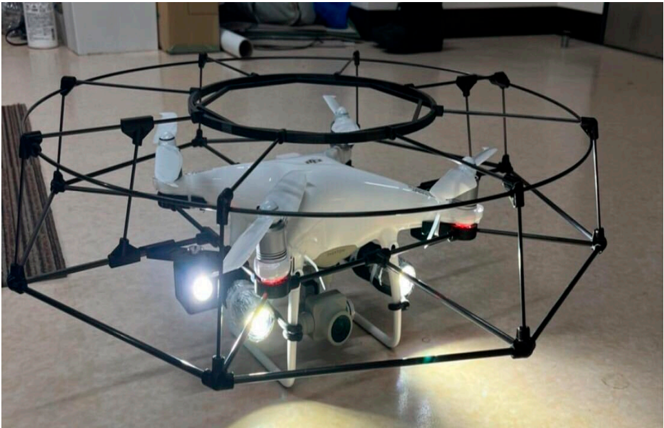
Figure 13. Drone system that can operate in underground inaccessible area with its cage.
