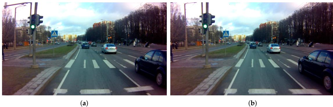
Figure 2. Comparing images obtained directly from the sensor to those that have been processed. (a) Raw distorted image obtained directly from the camera. (b) Rectified image.
