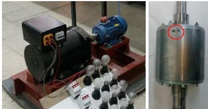
Figure 3. The experimental setup and the rotor with two broken bars.
