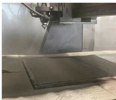
Figure 1. Spray deposition process of GNP coating on CFRP prepreg.
