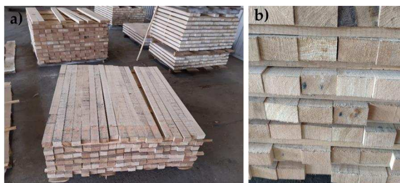
Figure 1. Sampling and sorting of green oak wood in the woodyard (a) and wax protection of the front and back ends before drying (b).
