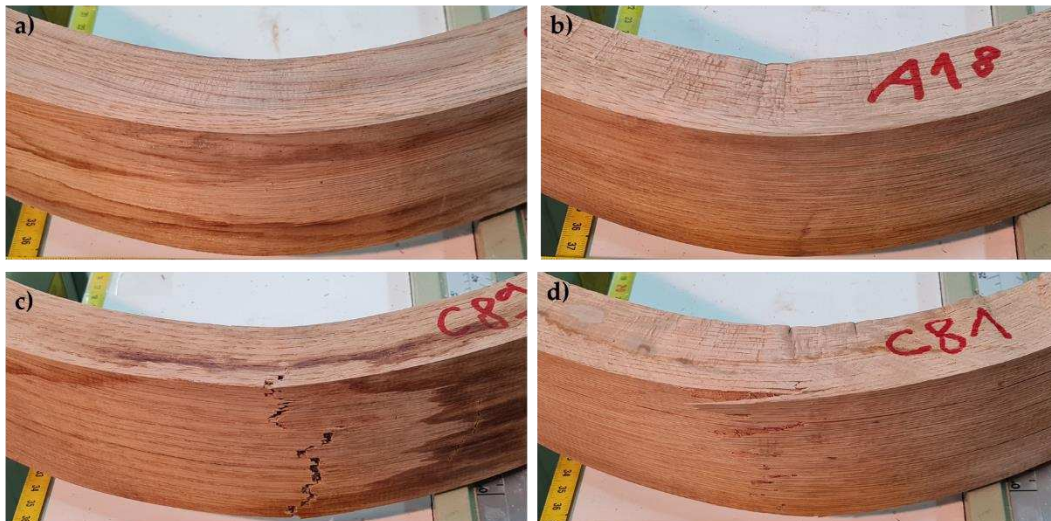
Figure 8. Visual assessment of defects on bent oak: a) no defects present, b) wrinkling, buckling and kneading of fibers on concave side (I – failure type), c) tensile brittle fibre break (II – failure type), d) buckling and kneading of fibers on concave side with additional tensile fibre break on convex side (III – failure type).
