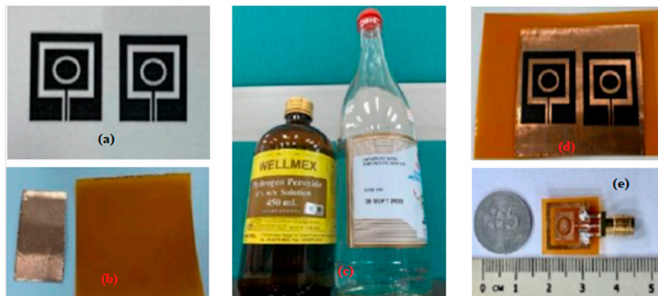
Figure 9. Fabrication Prototype (a) printed design (b) polyimide Kapton film with copper tape (c) chemical substances (d) designed transferred (e) complete prototype.
