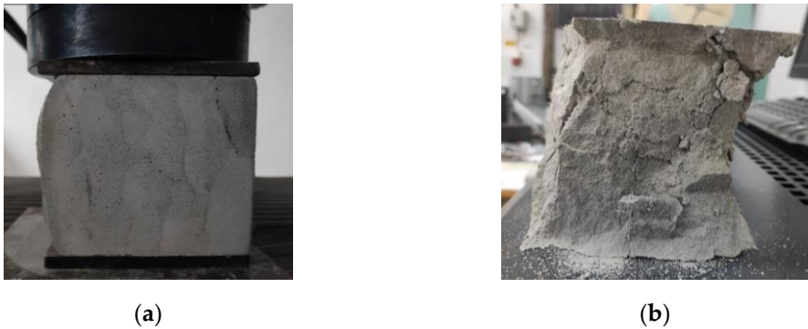
Figure 19. Specimen manufactured with M28 mix and printed with the 20 mm nozzle: (a) Set-up, (b) Failure mode
