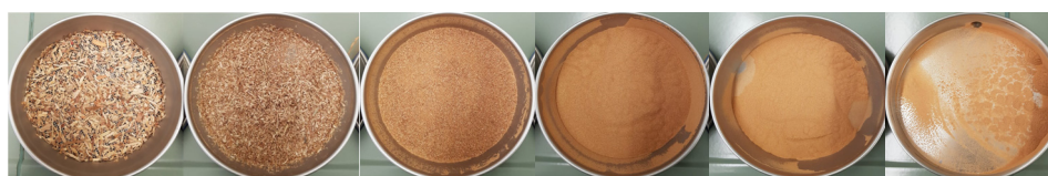
Figure 3. The sieves, from left to right: 2000, 630, 200, 112, 63 \mu\text{m} and the sieve-base with sawdust fractionated by electric sieve-shaker.
