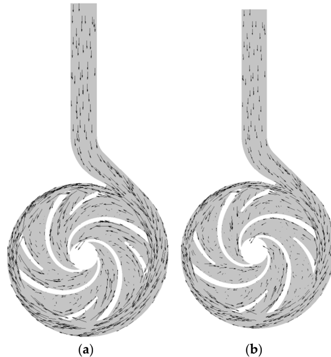
Figure 9. Velocity vector at Q = 12.5 \text{ m}^3/\text{h} (a) n = 1500 \text{ rpm} (b) n = 1750 \text{ rpm} .
