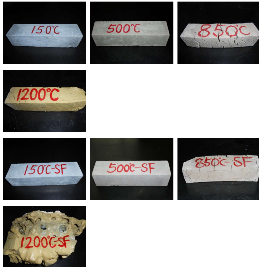
Figure 4. Apparent morphology of binders after heat treatment.
