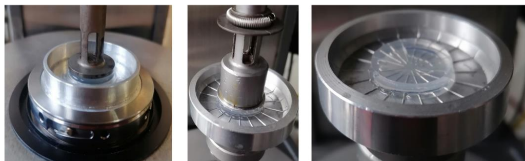
Figure 1. Photographs of the two plates geometry used for the gel rheology. The photograph on the left shows the smooth plate-plate mounted onto the Peltier system control. The photograph on the right shows the geometry of the radial ribbed plate. Both geometries have a diameter of 25mm consist of a cup on the bottom part and a plate on the upper part between which the gel is placed before being covered by a silicon oil to prevent evaporation of water.
