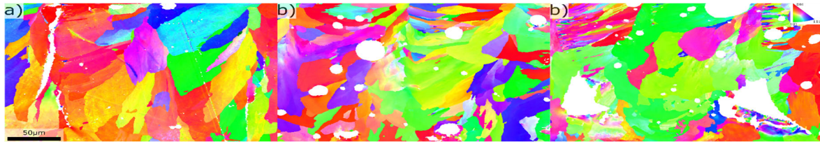
Figure 8. Grain structure for different alloy compositions, a) 0.2wt%Mg, 2.4wt%Si, b) 3.4wt%Mg, 1.5wt%Si c) 7.8wt%Mg, 2.4wt%Si.
