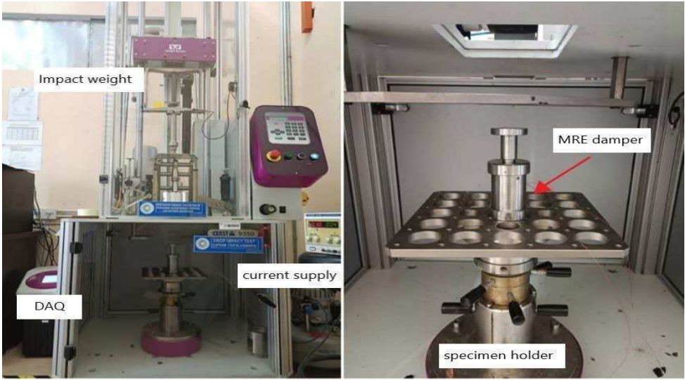
Figure 2. Drop Impact Test Machine used in this Study.
