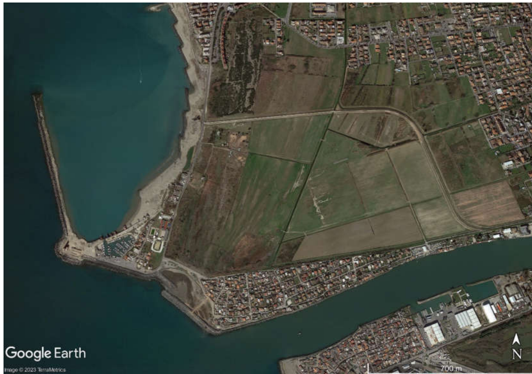
Figure 4. An aerial view of the embankment road reveals that the spontaneous settlement of Passo della Sentinella is not protected by the embankment. Protection is only provided for the built-up area to the north of the embankment. Source: Google Earth Pro.
