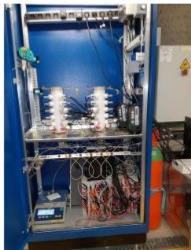
Figure 3. a. Schematic representation of the device within Underground Research Laboratory (URL) of ANDRA (Bure, France) with illustration of the circuit allowing supplying CO x pore water to the two Multi-Parametric Probe holders (MPPs). b. Cupboard (dimensions: 90×50×200 cm) with inside 2 MPPs & instruments (Computer, DAQ, pHmeters, flow controller, a precision balance connected to DAC). c. Outside of cupboard, a Potentiostat-Galvanostat, Impedancemeter.
