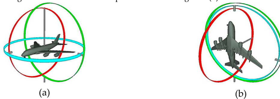
Figure 5. An example of the gimbal lock problem. The aircraft has lost one of the degrees of freedom (b) - in this case the ability to roll. The aircraft in this case will stall.
