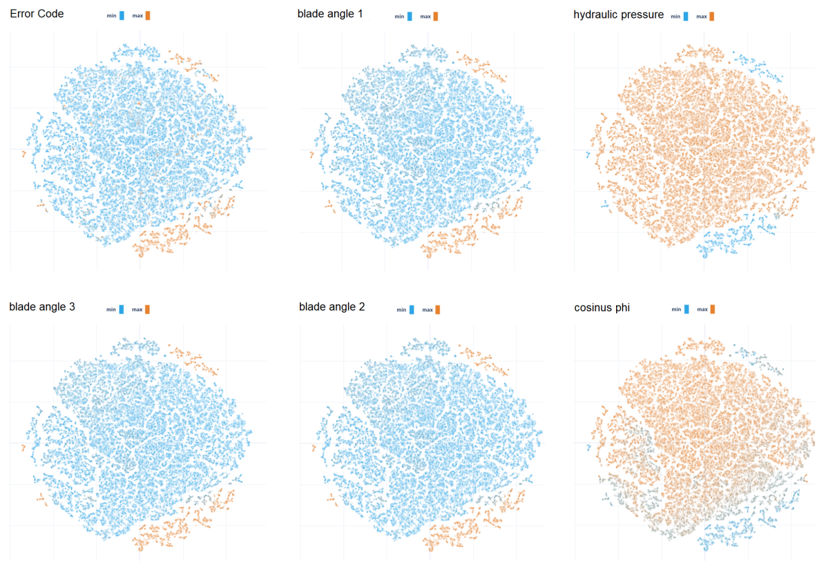
Figure 12. T-SNE projection of error codes and inputs into a 2D space. The error codes cluster well in a few distinct regions and some inputs show high correlation to these clusters. However, all inputs that were identified by this method are consequences of a gearbox failure not a cause.
