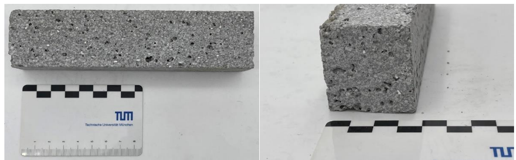
Figure 14: Post-processed specimen (20 mm) before strength tests. Few voids and imperfections.
