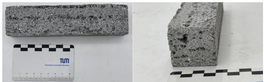
Figure 15: Post-processed specimen (80 mm) before strength tests. Major voids and imperfections.
