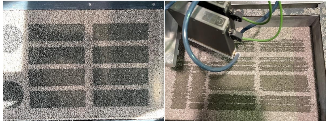
Figure 12: Cement paste distribution at 20 mm Figure 13: Cement paste distribution at 80 mm
