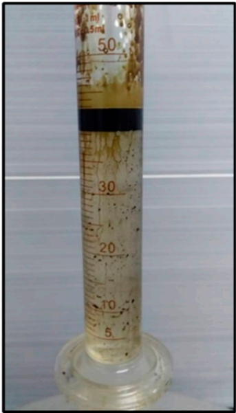
Figure 17. Oil extracted after water and polymer flooding at 60 °C. The polymer solution is consisted from 2000 ppm HPAM and 0.8 wt.% CSNPs.
