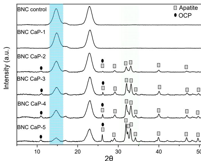
**Figure 6.** Phase analysis of the diffractograms of the biomineralized NCB microporous 3D scaffolds.
