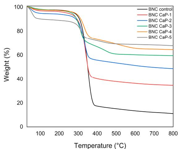
**Figure 4.** Results of thermogravimetric analysis of biom mineralized BNC microporous 3D scaffolds. An unmodified BNC microporous 3D scaffold was used as a control.
