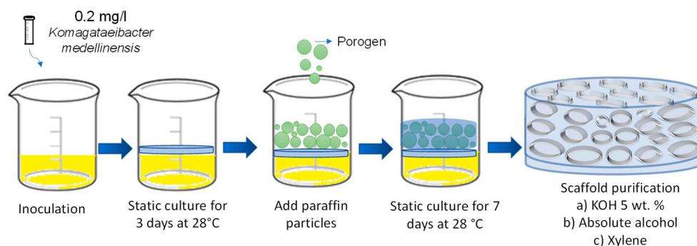
**Figure 1.** Schematic illustration for the design of microporous 3D scaffolds of bacterial nanocellulose.
