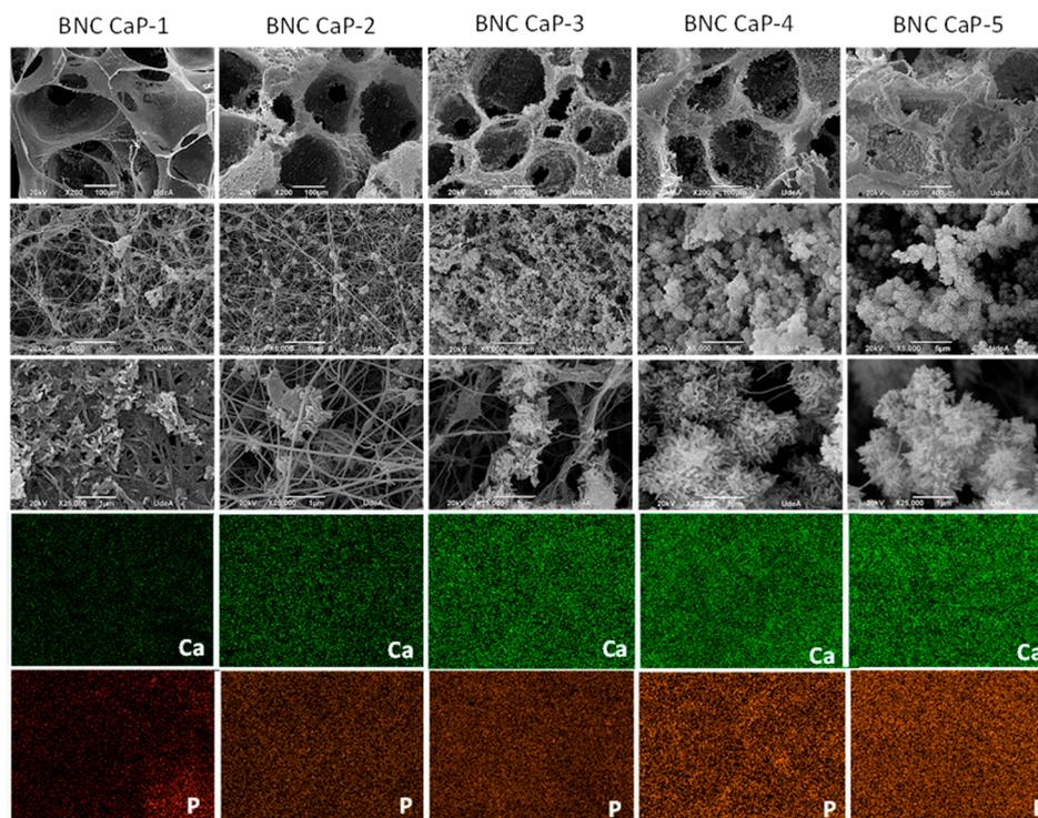
**Figure 3.** Electron micrographs taken by SEM at 200x, 5000x and 25000x (rows 1 to 3) and elemental maps made by EDS with a scale of 10  $\mu\text{m}$  (rows 4 and 5) of the microporous 3D scaffolds of biom mineralized BNC. From left to right column 1: BNC control, column 2: BNC cycle 1, column 3: BNC cycle 2, column 4: BNC cycle 3, column 5: BNC cycle 4, and column 6: BNC cycle 5.
