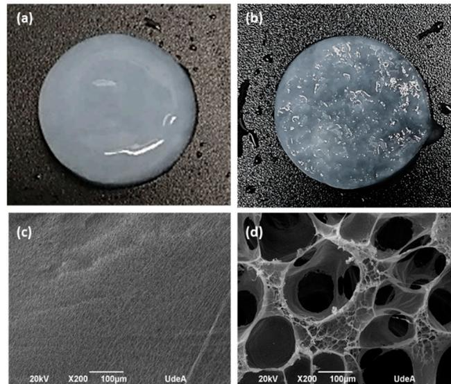
**Figure 2.** Scaffold morphologies a) photograph and c) micrograph taken by SEM of BNC membrane used as control; b) photograph and d) micrograph taken by SEM of microporous 3D BNC scaffold.
