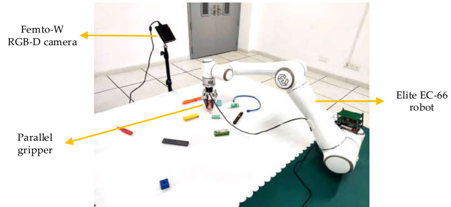
Figure 10. Physical experiment conditions. Experiment instruments include a Femto-W RGB-D camera, an EC-66 collaborative robot, a parallel gripper and some objects to be grasped.
