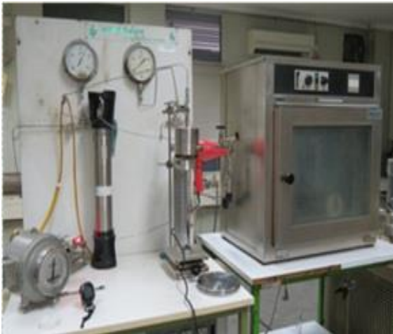
Figure 8. MMP determination apparatus in laboratory using slimtubes
