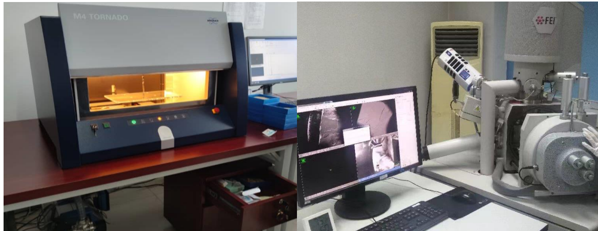
Figure 4. (a) Micro-XRF spectrometers M4 Tornado, (b) Scanning Electron Microscope.
