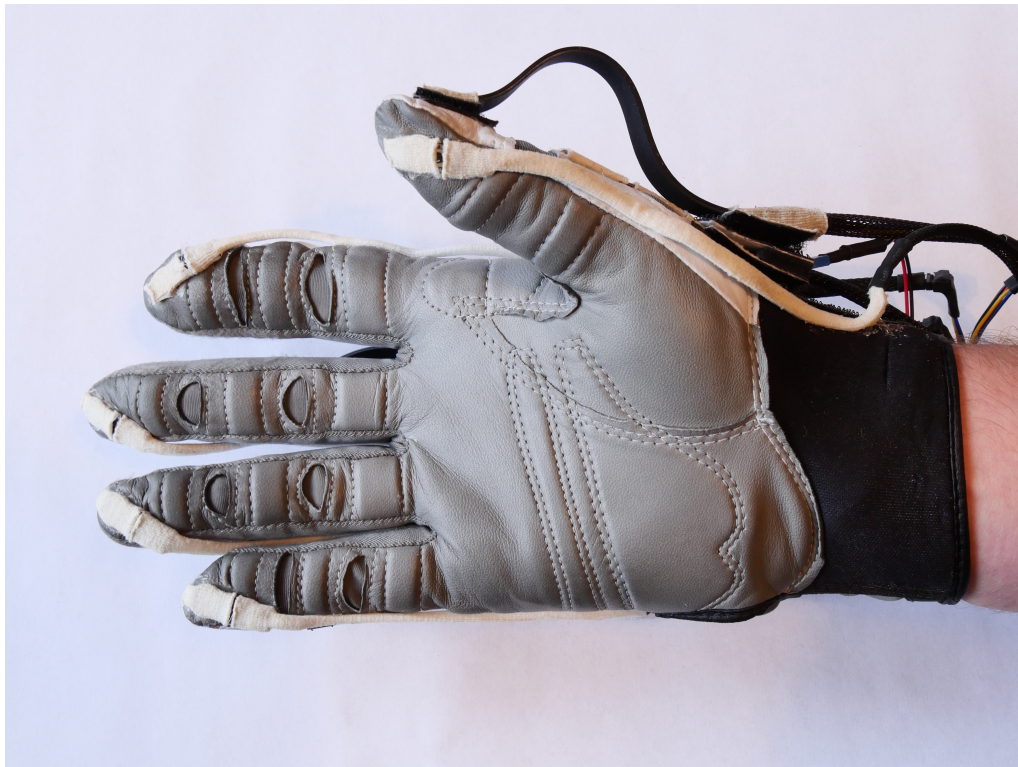
Figure A9. SenGlove in palmar view. Realization shown for a medium-sized right hand with all five fingers equipped with sensors.
