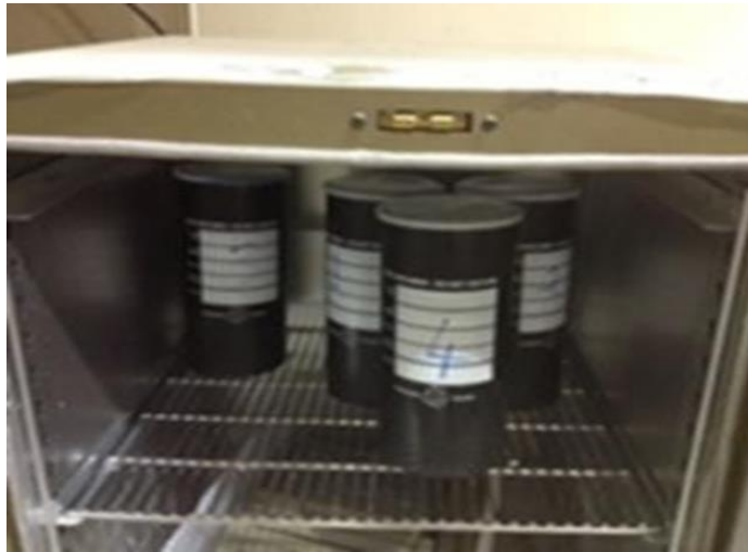
Figure 7. Mortar bar storage for AMBT testing
