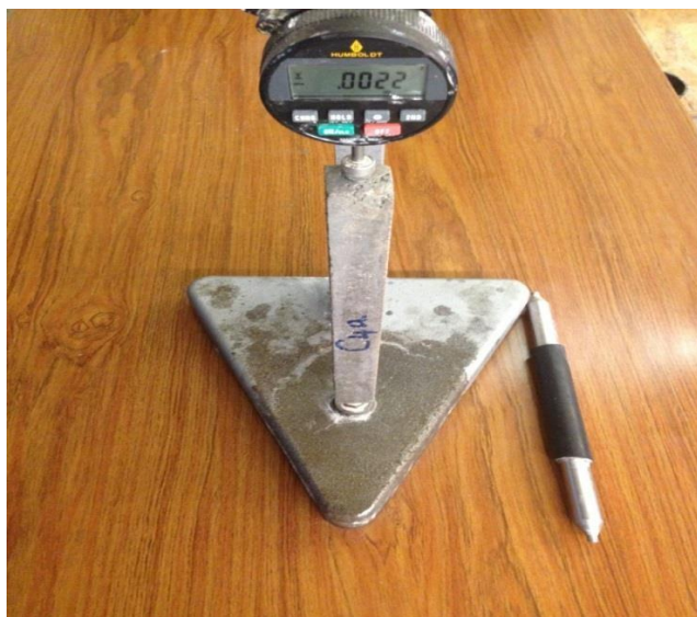
Figure 8: Mortar bar expansion measurement (using standard metal bar comparator)
