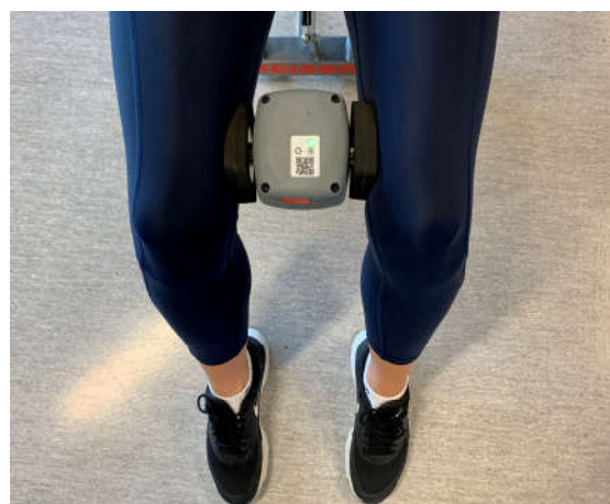
Figure 3. Strain gauge affixed to rack using push plates.
