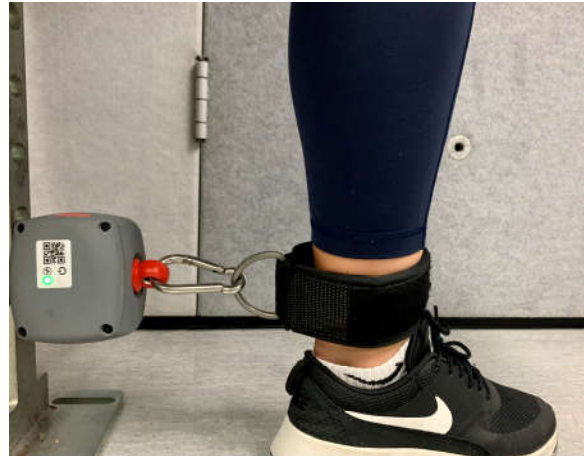
Figure 4. Strain gauge affixed to rack using ankle strap.
