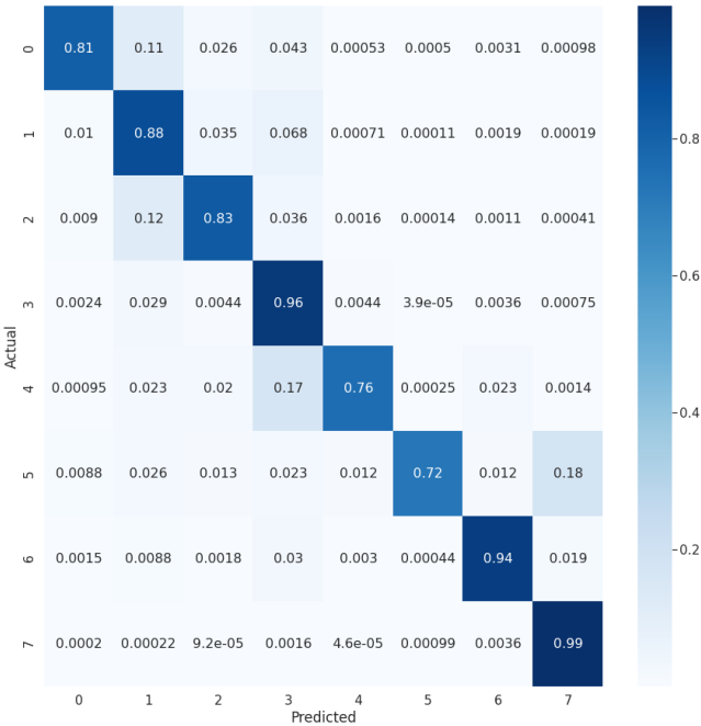
Figure 8. Normalized confusion matrix for the segmentation in 8 classes with U-Net.
