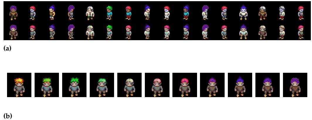
Figure 6. Results on Sprite dataset. (a) Comparison between input sprite images (first row) and reconstructed ones (second row). (b) Images generated fixing all the latent variables' dimensions but one, which is varied. Generated sprites have fixed attributes but continuously varying hair style.
