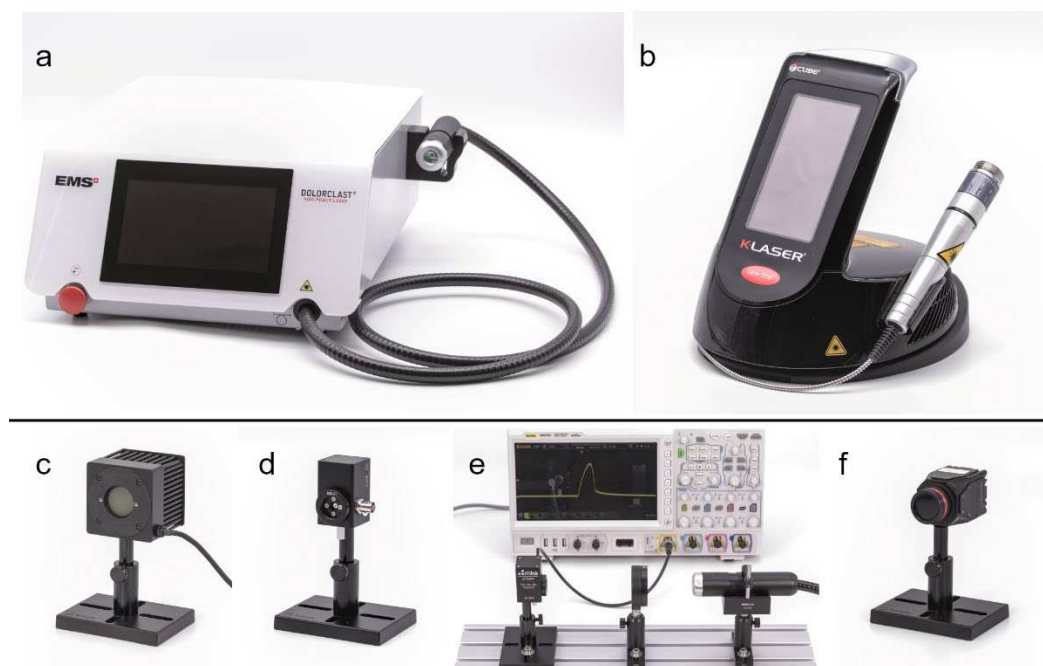
Figure 1. Laser therapy devices and sensors used in the present study to investigate laser beam parameters: (a) EMS laser; (b) K-laser; (c) thermal power sensor; (d) photodiode; (e) experimental
