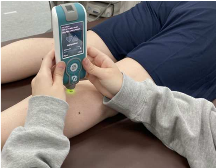
Figure 3. Mechanical property measurement using MyotonPRO.
