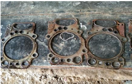
Figure 1. Damaged cylinder head gasket.
