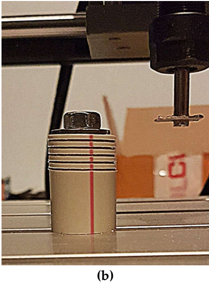
Figure 8. Technological sketch (a) and photograph (b) of milling a special thread on a CNC 3018 Pro machine.
