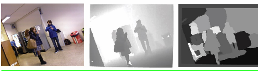
Figure 2. Raw color image (left), depth map (middle), and segmentation map (right).
