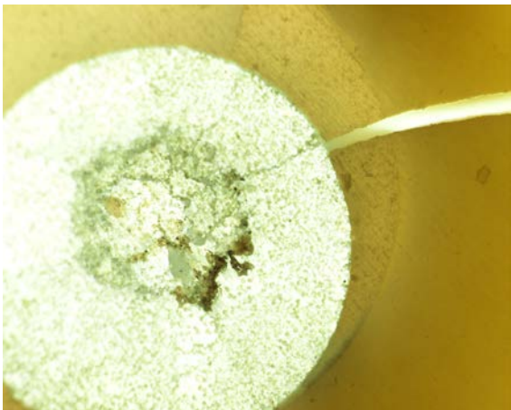
Figures 1E Group 5: Cohesive failure of a fiber post.
