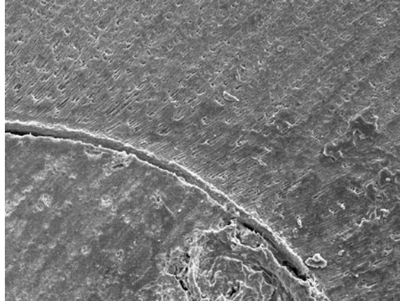
Figures 2B Group 2: no resin tags (G-Premio Bond) are visible and adhesive failure type (SEM x200).
