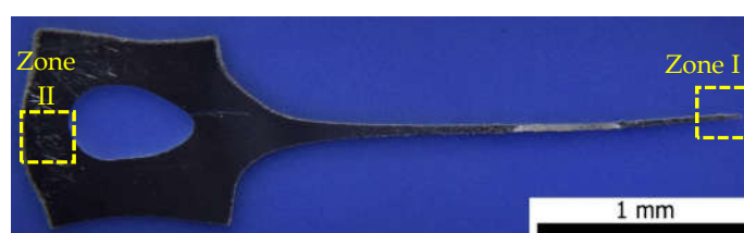
Figure 1. General view of the UFG aluminum alloy No. 6 specimen after superplasticity tests at 450 °C, 3.3 \cdot 10^{-2} s ^{-1} . Studied areas are indicated with dash lines.
