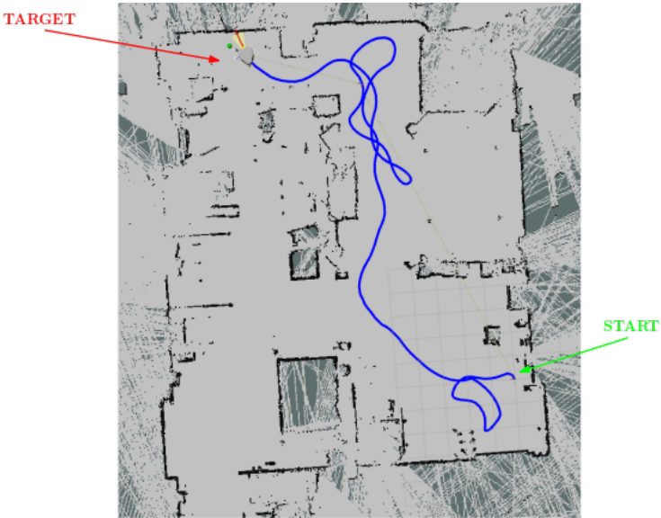
Figure 18. Trajectory of the robot for the point to point motion in presence of moving pedestrians as dynamic obstacles.
