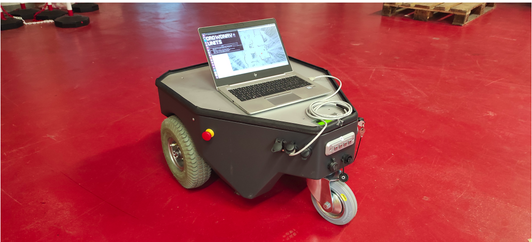
Figure 15. The elected differential drive mobile robot used in the experimental campaign: a Neobotix MP-500.
