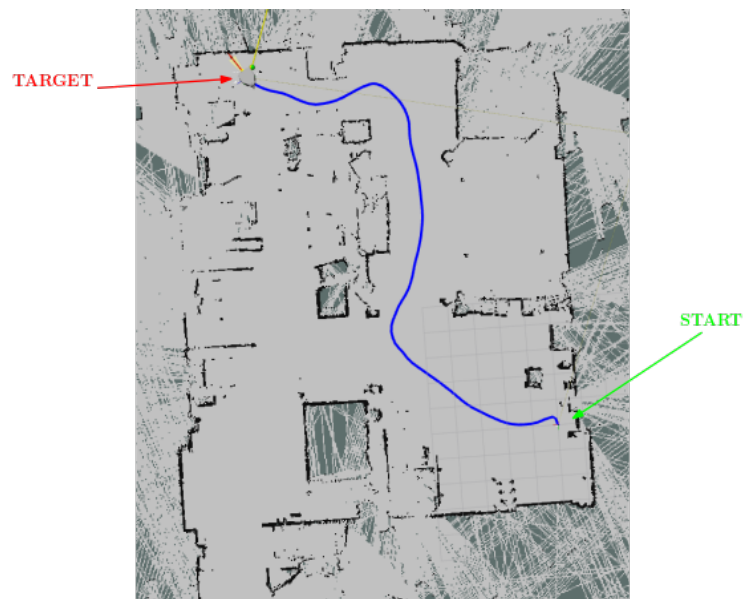
Figure 16. Trajectory of the mobile robot for the point-to-point motion in the absence of dynamic obstacles.
