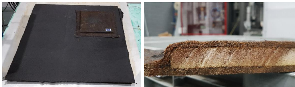
Figure 12. Size comparison between the demonstrators for industrial purposes (1 m 2 ) and for material characterization (0.16 m 2 ) (left); Sandwich structure linseed-PET-linseed (right)
