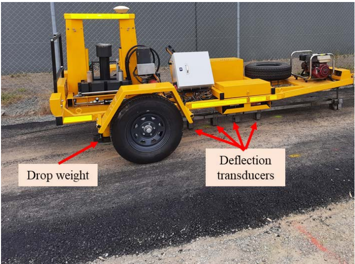
Fig. 6 FWD test on compacted asphalt layer.
