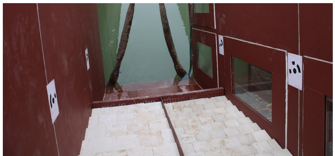
Figure 27. Detail of the perforated metal plate, where the downstream row of the WSB was supported
