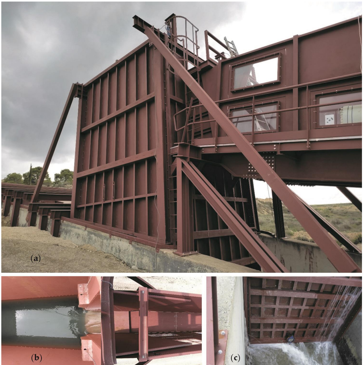
Figure 5. (a) General view of the supply tower (b) Photographic montage of the water inside the supply tower (left) exiting towards the test chute (right). (c) Wall gate of the supply tower and 250-mm diameter butterfly valve to facilitate its manoeuvre by emptying the water retained upstream.
