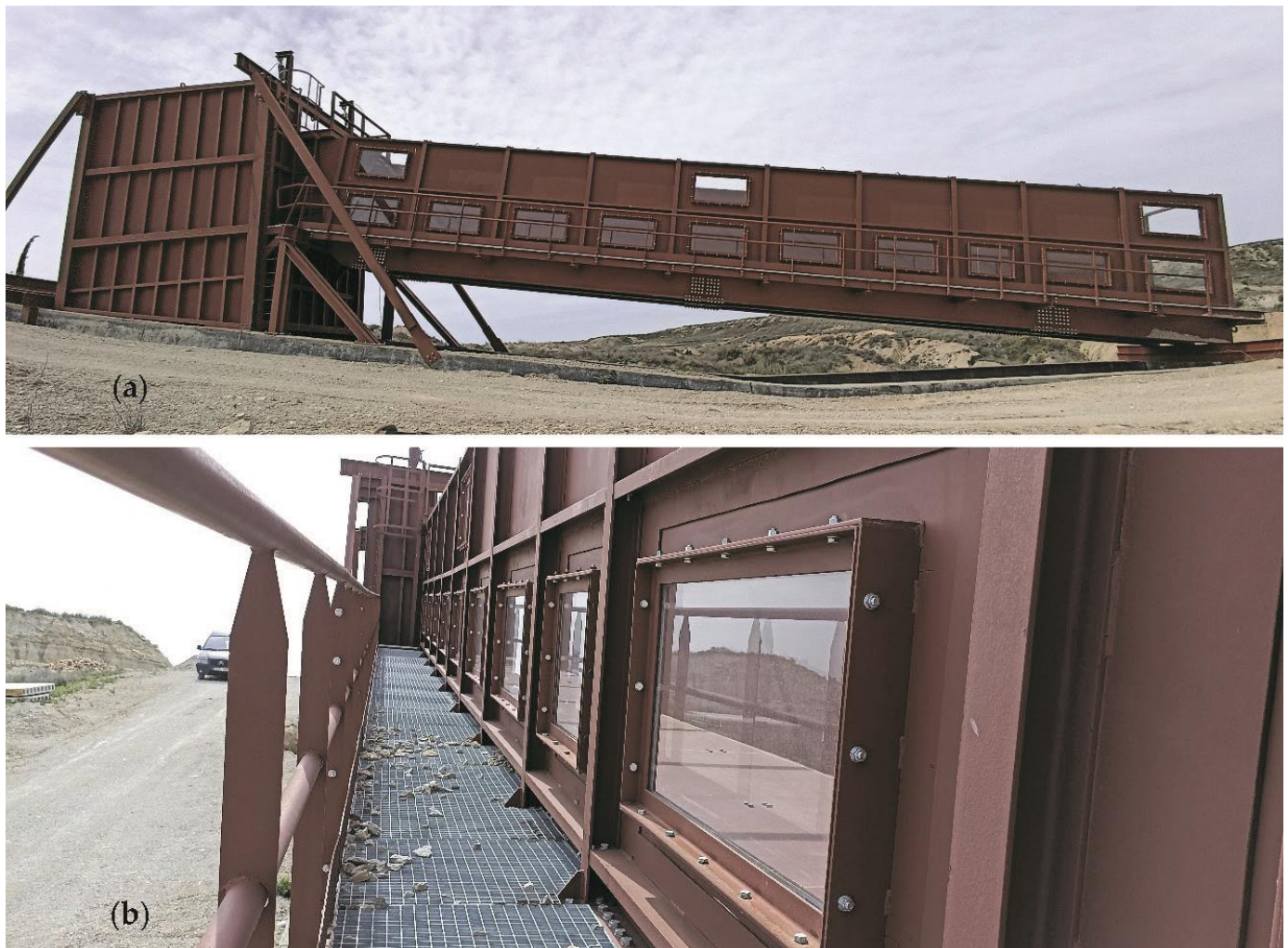
Figure 6. (a) General view from the right bank of the test chute before being lowered to the bottom of the auxiliary channel (b) Photo of the inspection windows from the side platform of the chute. In the background, the supply tower.
