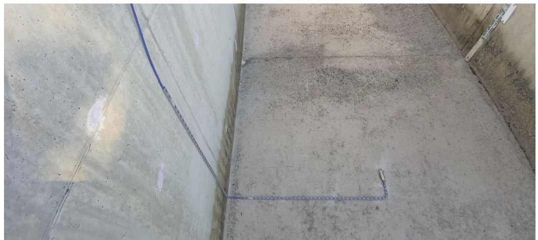
Figure 14. Picture of the sensor of the Nivus Portable Flowmeter installed in the centre of the auxiliary channel, upstream of the testing chute.
