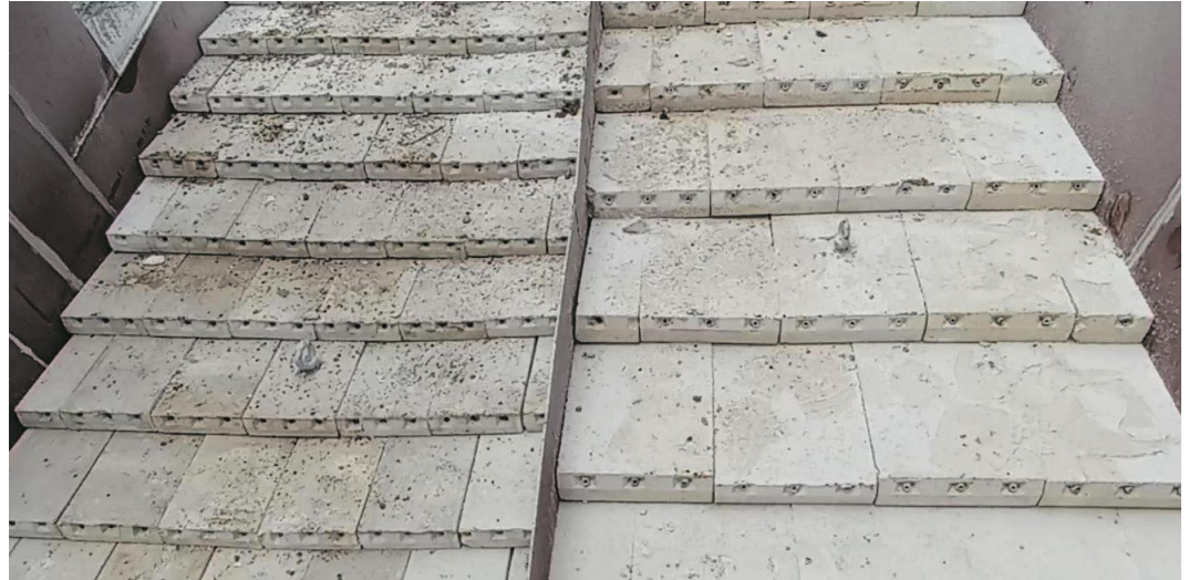
Figure 13. Photo of two eyebolts installed on some of the WSBs for block-extraction tests.
